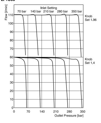
All characteristic curves measured with HLP46 at 50 °C.
