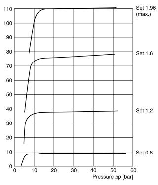
All characteristic curves measured with HLP46 at 50  $^{\circ}\text{C}.$
